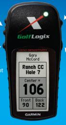
Page Button Press to select between multiple courses. Press and **Hold for 4 Seconds** to Check Battery Signal and Adjust Screen Contrast
